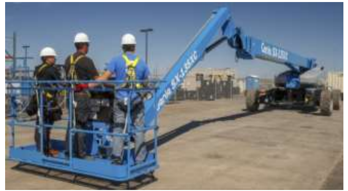
MOBILE ELEVATED WORKING PLATFORM MACHINE FUNCTIONAL TESTING
