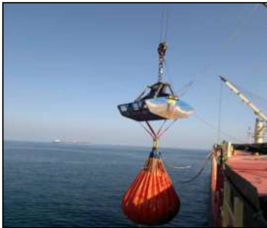
LOAD TEST OF GRABS ON BOARD VESSEL "HYDERABAD"
