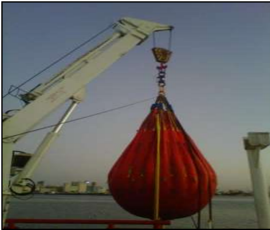
LOAD TEST OF DECK CRANE VESSEL "ONBOARD OFFSHORE SUPPORTER"
