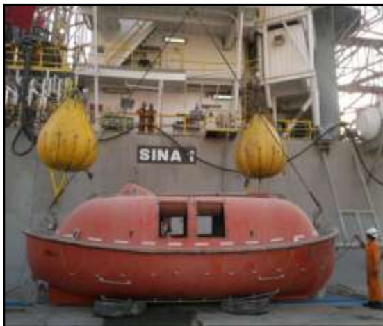
LOAD TEST OF GRAVITY TYPE LIFEBOAT DAVITS ONBOARD OILRIG "SINA1"
