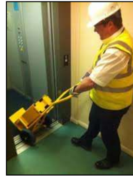
ELEVATOR LOAD TESTING
