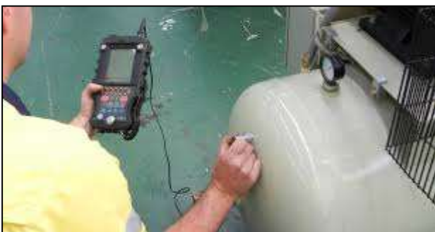
AIR RECEIVER THICKNESS TESTING
