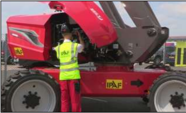
MOBILE ELEVATED WORKING PLATFORM MACHINE VISUAL EXAMINATION
