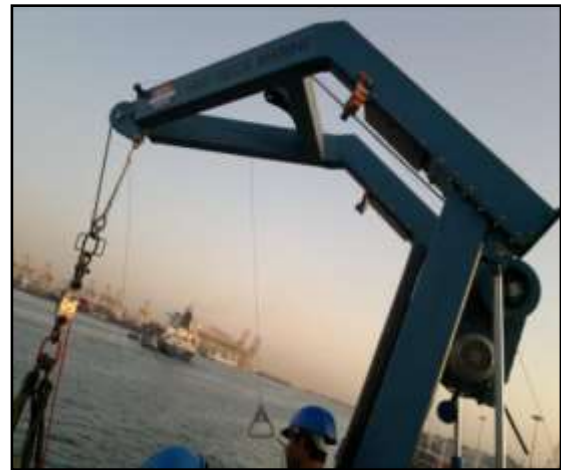
LOAD TEST OF FRC DAVIT- USING CALIBRATED LOAD CELL & WATER BAG.
