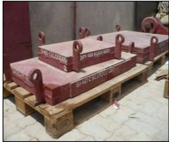
VARIOUS CALIBRATED TEST WEIGHTS - 200, 500 & 1250 KGS, etc
