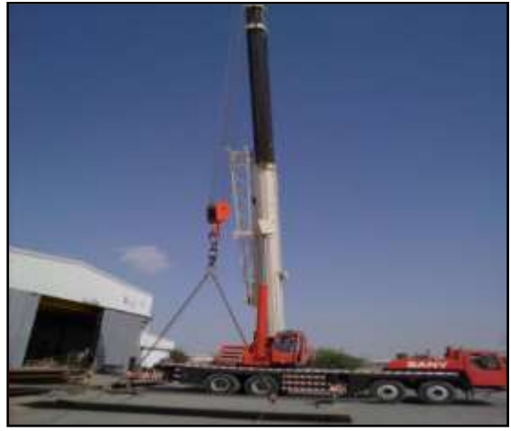
LOAD TEST OF MOBILE CRANE - USING CALIBRATED TEST WEIGHTS & LOAD CELL.
